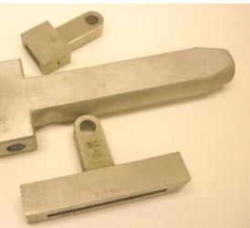
**Machine Holders** – There are various configuration of holders available to suit the different applications and the length of slot determines the number of individual pieces of type that can be inserted. Any length of slot not used by type is filled using spacing pieces.
