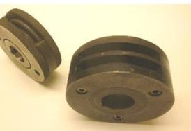
**Rotary Holders** – Uses wedged (segmented) type to efficiently mark flat or round surfaces. This type of holder is commonly used in the packaging industry.
