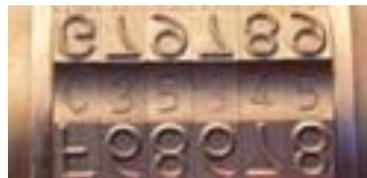
Numbering units with 1.5mm to 3mm characters can be fitted with interchangeable shanks for hand or machine use. Standard engraved wheels are 0-9 with one blank station. Wheels with letters, symbols or repeated characters are available by quote.
